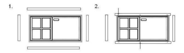
Insert door frame in to its space from the outside of the structure. Then fix the rest of the support trims from inside the building:
