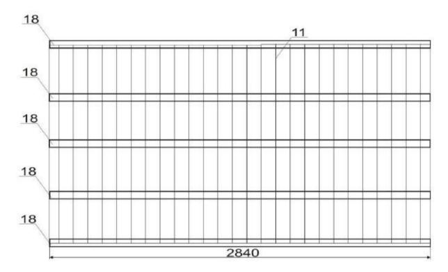
4.4. Assembling the walls: place the wall-boards on the bearers as shown in a general sample below:
