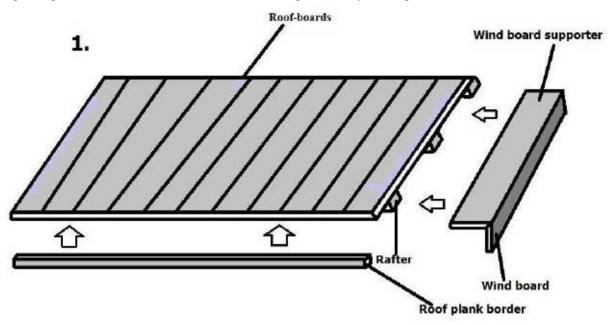
Attach the roof plank border to the roof boards ant screw in the roof plank on top.
